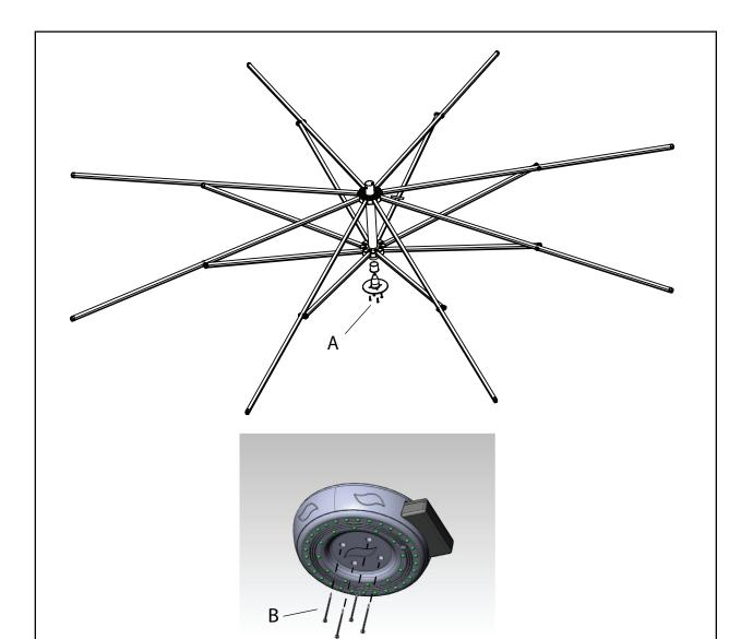
**Step 1:** Remove (4) #6 x 1/2" screws at the base of the Umbrella Cage (A).
