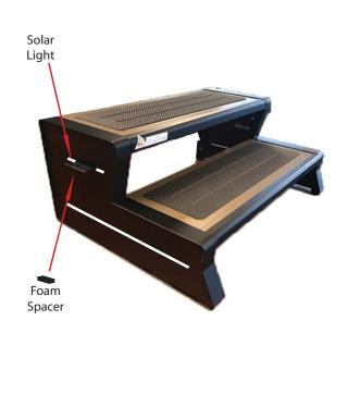
**Step 1:** Slide the ModStep solar light panel throught the slot in the ModStep riser from the inside.
