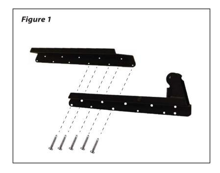
Attach the CMIII Eco Extender Bracket in between the CMIII Eco Bracket and the Spa using the provided #10 x 1" Mounting Screws. Note: At least 5 mountings screws must be used to attach the CMIII Eco Bracket to the CMIII Eco Extender Bracket.
