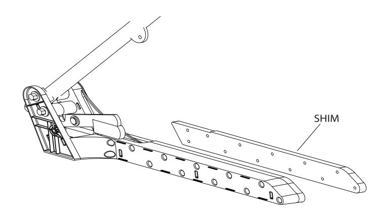
**Step #1**Mount your CMIII Shim in-between the Spa Skirting and the CMIII Bracket using the supplied #12 x 2-1/2" screws.
